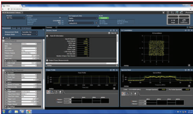
▲ Fig. 4 Measured Tx power, EVM, signal constellation, spectral mask and power profile.
